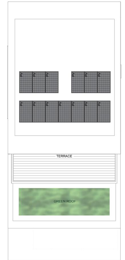
13 x 300KW Solar PV System Panels
